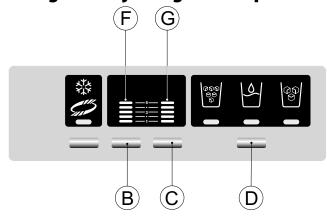
To adjust the refrigerator temperature, press button C. The indicator (G) will illuminate. Each subsequent press of button C will adjust the temperature scale by one. To clear the setting, simply keep pressing button C until indicator (G) is back to level 1.
